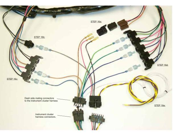
Adaptation of original "Sweep Dash" harness to accept disconnect plugs from new Instrument Cluster Harness.
