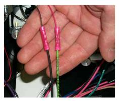
This is a completed LED splice for the high beam indicator.
